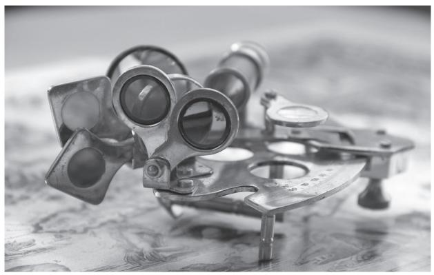
A sextant is an instrument for calculating latitude and longitude. It is based on trigonometry: the earth is a giant circle, and the angular position of the sun (or a given star) above the horizon defines the necessary triangle.
